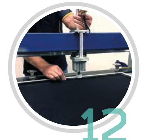
Engage beads to the groove in the frame. Compress the beads into the frame using the Ulltrasafe Assembly Machine,
